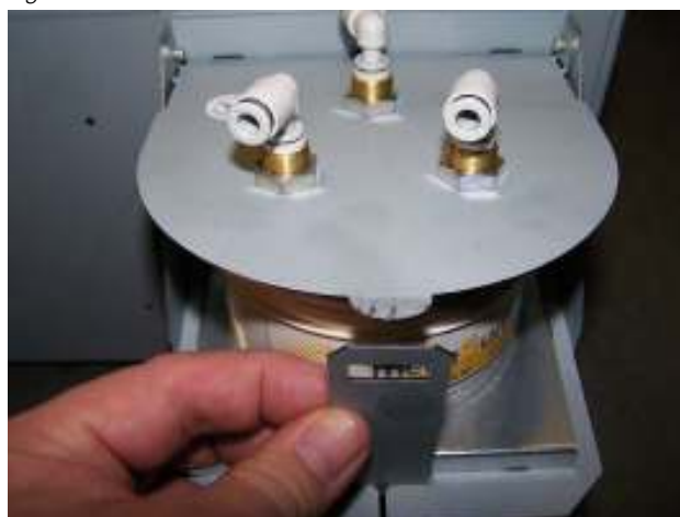
Figure 51.1 Latch of the Aroma tin
