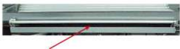
Figure 47.2: Filter pad in the base section
