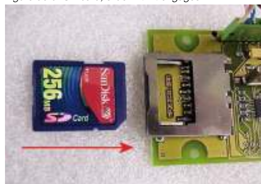
Figure 50.5: SD card; slide in till it engages
