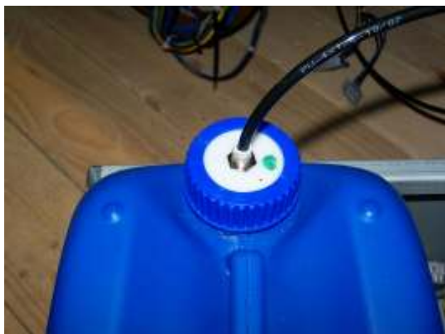
Figure 52.1 Hose connection on aquaCool canister
