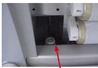
Figure 47.4: Tensioning spring on the right-hand side
