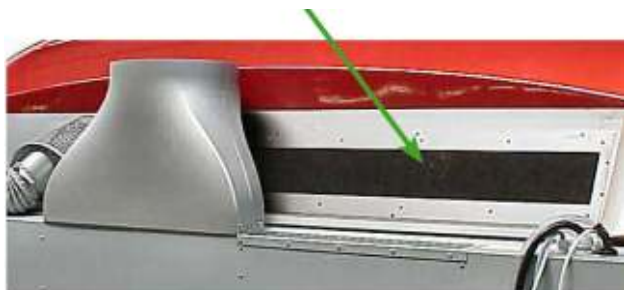
Figure 47.1: Filter pad in the canopy
